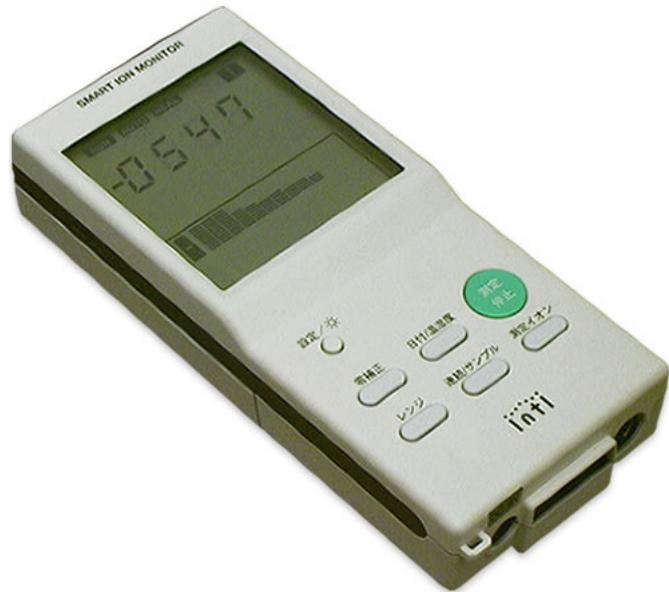
The Air Ion Counter (or A.I.C. as its more commonly referred to) is a handheld device that's designed to measure ion density. The counter is used in a number of scientific fields and specifically measures the number of ions (both positive and negative) per cubic centimeter or the average in a given area. In paranormal investigation and research the device is used as a gauge which can measure paranormal activity and sometimes the direct (though unseen) presence of a ghost or entity.
