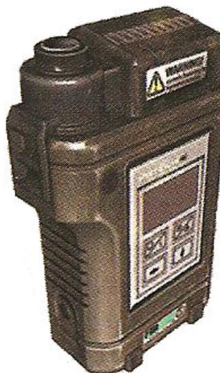
**K-9 Material Sampler:** This handheld device was designed as a simple “point and shoot” tool to assist in determining the makeup of specific substances to help expedite crime scene investigating and forensics. Sampler must be used within three feet of the trace evidence desired to be analyzed. Note: Oftentimes the use of the *UV light* and/or the *Laser Light pointer tool* will be helpful in discovering trace evidence to analyze.
